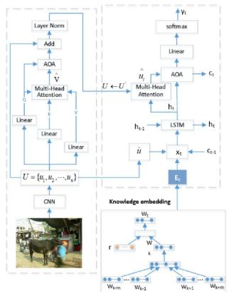
The KE-AoA model applies the AoA module to the image encoder and combines knowledge embedding with the decoder. By combining semantic features from refining knowledge representations with visual features of the image, our model can better model relations among different objects and generate more accurate captions.
